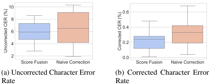
Fig. 9: Box plots depicting mean, median and quartiles of the participants' performance including corrected and uncorrected character error rates under the two conditions.
